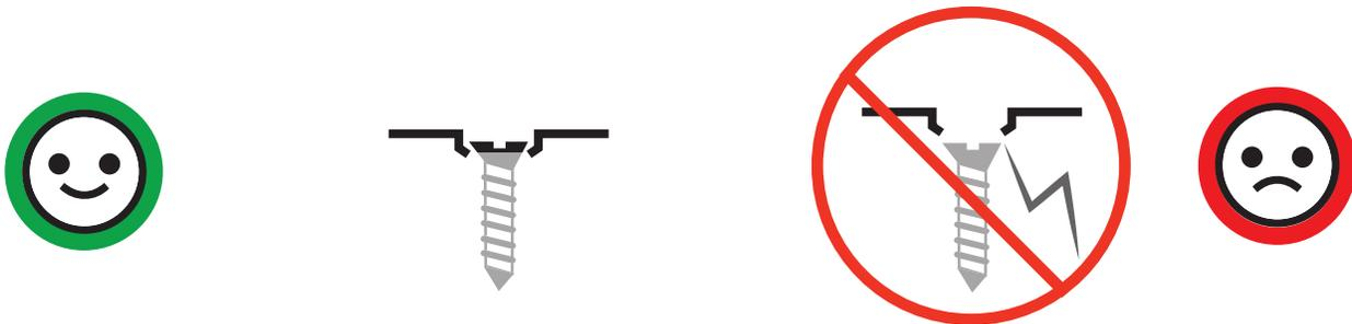
To complete assembly, use hand-held screwdriver to fully tighten all screws until they're snug.
