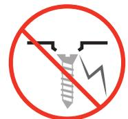
**DO NOT** use power tools to assemble. Using power tools will cause product to crack!
